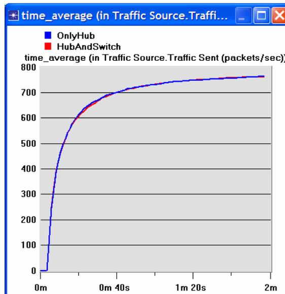
4. Select the **Traffic Received (packets/sec)** statistic and click **Show**. The resulting graph should resemble the one below. As you see, the traffic received with the second scenario, **HubAndSwitch**, is higher than that of the **OnlyHub** scenario.
