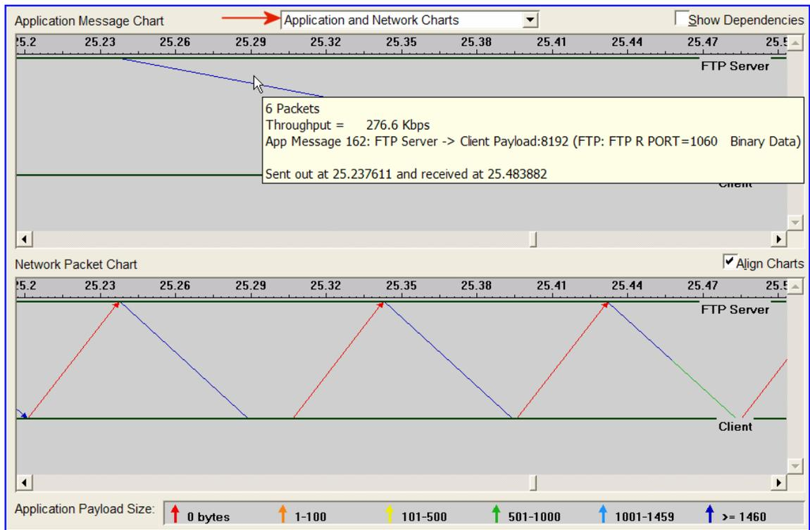
The Network Chart shows that this application message causes many packets to flow over the network. These packets are a mix of large (blue and green) packets from the FTP Server to the Client and small (red) packets from the Client to the FTP Server. As the red color indicates, these packets contain 0 bytes of application data. They are the acknowledgments sent by TCP.
