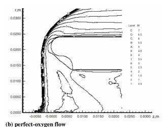
Fig. 11. Mach number contours in oxygen flow about a toroidal ballute model at  $Kn_{\infty D} = 0.005$ .
