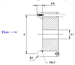
Fig. 9. The ballute model used in experiments [17].
