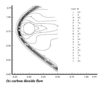
Fig. 2. Mach number contours in flows of argon and carbon dioxide about a torus at  $Kn_{\approx D} = 0.01$ ,  $M_{\infty} = 10$ , and H/R=8.
