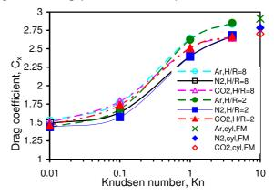
Fig. 8. Drag coefficient  $C_x$  of a torus vs. Knudsen number  $Kn_{\bowtie D}$  and various geometrical factors H/R in argon, nitrogen, and carbon dioxide at  $M_{\infty} = 10$ .
