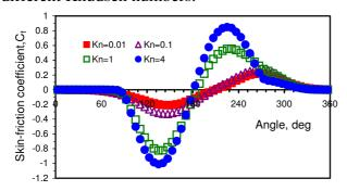
Fig. 6. Skin-friction coefficient  $C_f$  along the torus surface in nitrogen flow at H/R = 2,  $M_{\infty} = 10$ , and various Knudsen numbers  $Kn_{\infty D}$ .
