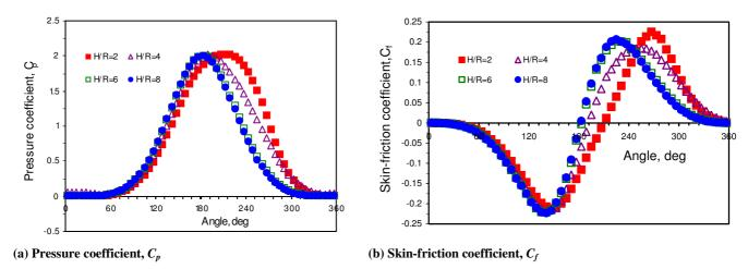
Fig. 4. Pressure and skin-friction coefficients along the torus surface in nitrogen flow at  $Kn_{\infty D} = 0.01$ ,  $M_{\infty} = 10$ , and various geometric factors H/R.
