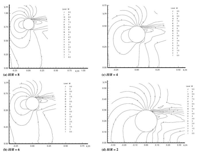
Fig. 5. Mach number contours in nitrogen flow about a torus at  $Kn_{\infty D} = 1$ ,  $M_{\infty} = 10$ , and various geometrical factors H/R.
