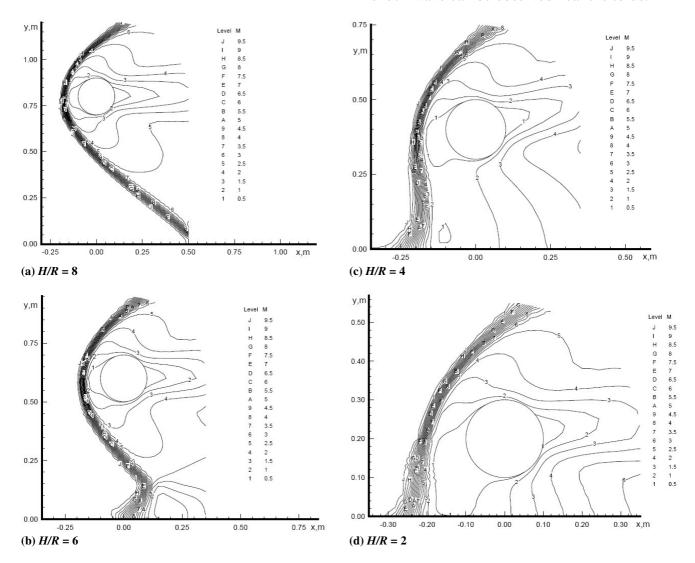
Fig. 1. Mach number contours in nitrogen flow about a torus at  $Kn_{\infty,D}=0.01$ ,  $M_\infty=10$ , and various geometrical factors H/R.
