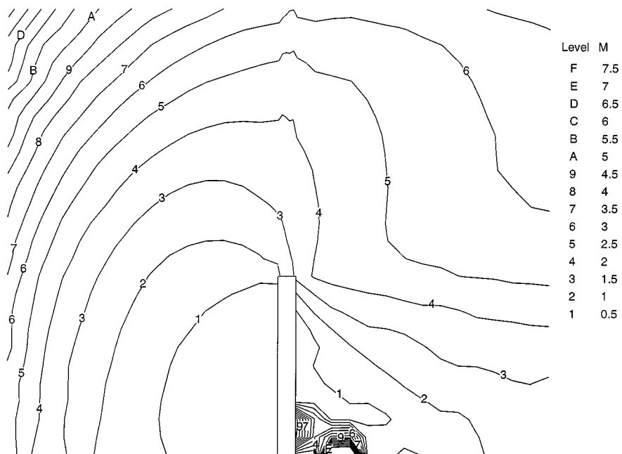
Fig. 9 Mach number contours in argon flow near a disk ( \alpha = 90 deg) at Re_0 = 10 , M_\infty = 10 , and t_w = 1 .
