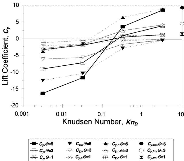
**Fig. 1** Lift coefficient  $C_y$  of a spinning cylinder vs Knudsen number  $Kn_D$  at  $M_\infty = 0.15$  and different spin rates: filled symbols,  $\Theta = 6$ ; open symbols,  $\Theta = 3$ ; and crossed symbols,  $\Theta = 1$ .
