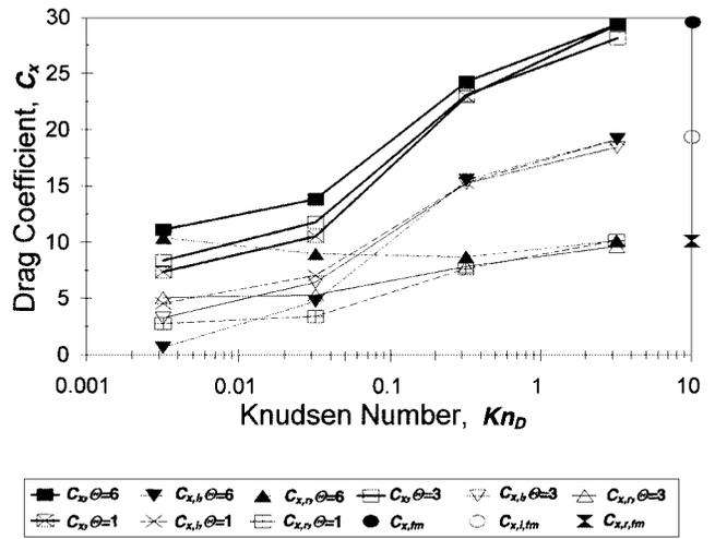
**Fig. 2** Drag coefficient  $C_x$  of a spinning cylinder vs Knudsen number  $Kn_D$  at  $M_\infty = 0.15$  and different spin rates: filled symbols,  $\Theta = 6$ ; open symbols,  $\Theta = 3$ ; and crossed symbols,  $\Theta = 1$ .
