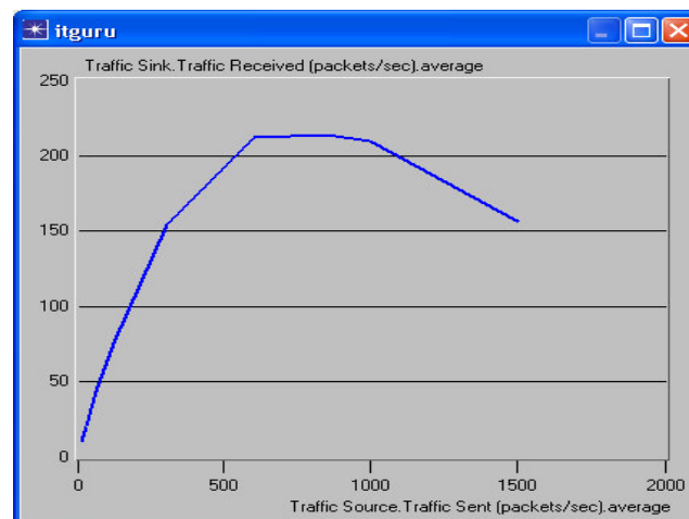
Fig. 1. Traffic received (throughput) vs. Traffic sent (load).
