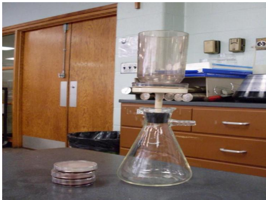
Figure 1. Filtering apparatus for the membrane filtration technique.
