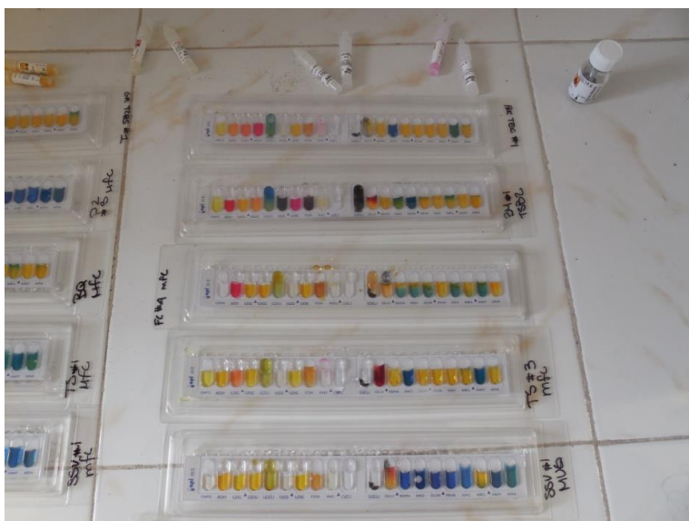
Figure 4. Scoring inoculated API 20E microbial identification strips after 18-24 h incubation.
