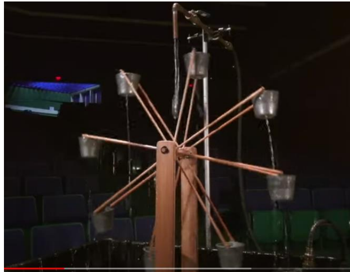
Figure 6. The Chaotic Waterwheel settings made by the Harvard Natural Sciences Lecture Demonstrations group [R15].
